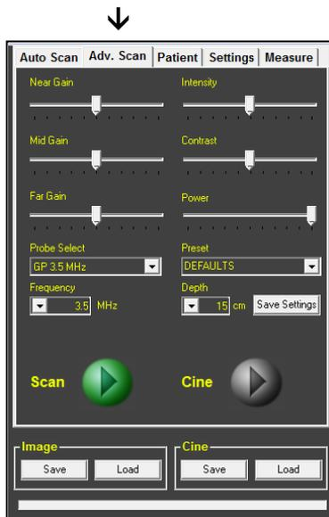
In the right hand column of sliders you can adjust the **Intensity** and **Contrast**. Typically you will leave these in the center. **Power** controls the probe's pulse power. Typically, **Power** will be at the maximum unless the image is saturated with the **Gains** centered.
