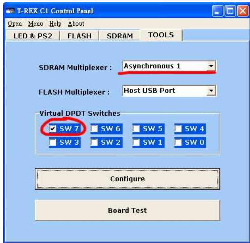
Figure 7.2 Need to activate SW7 with SDRAM R/W port set to Port 1 to listen to the music played
