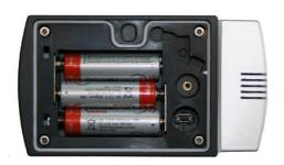
Insert three fresh AA alkaline batteries in the battery compartment. Be sure to observe the polarity.
