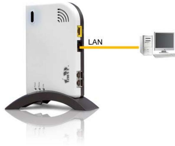
2. Set your IP address in local area network of computer as **Obtain an IP address automatically**.
