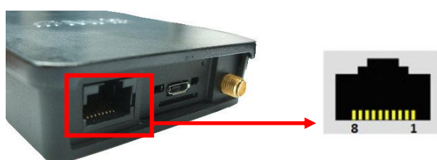
Figure 5: RJ45 Connector Pin Definition for MLB-G3002
