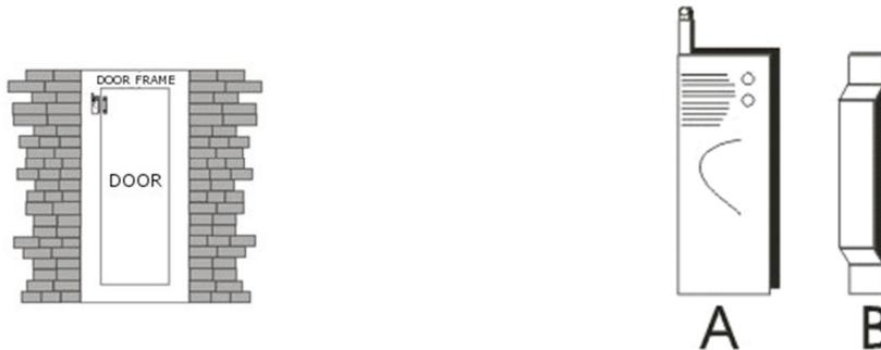
1. The surface for door sensor installation should be clean so door sensor can be attached to the door and frame firmly with double faced adhesive.
