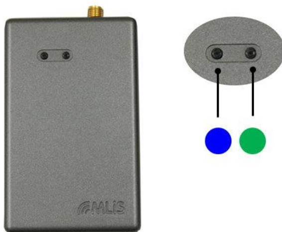
Figure 6: LEDs for MLB-S-BGS2-BW
