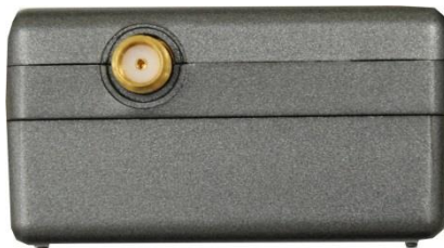
Figure 4: Antenna Connector for MLB-S-BGS2-BW
