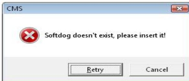
Watchdog error may be caused by watchdog drive not installed, watchdog inserted improperly, or USB port damaged. Please check watchdog driver or reinsert watchdog.
