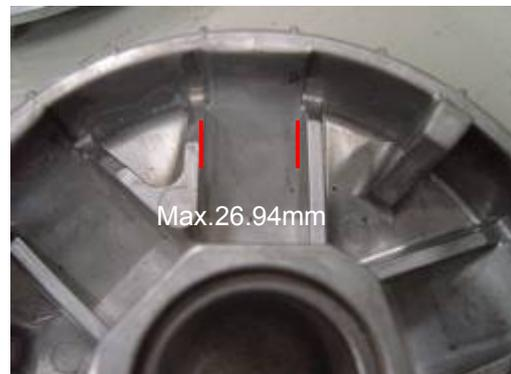
Check the driver face for wear or damage.
