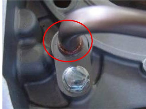
Install the crankshaft into the left crankcase being careful not to damage the oil seal.
