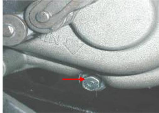
Remove drive sprocket.
