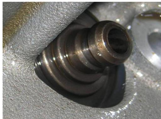
Subtract each valve stem O.D. from the corresponding guide I.D. to obtain the stem-to-guide clearance.
