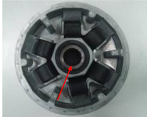
Apply grease to the drive pulley collar.
