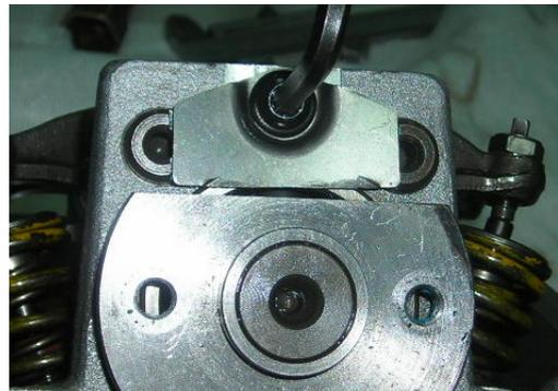
Push the cam chain adjuster push rod back into the adjuster body by pressing the tab down.
