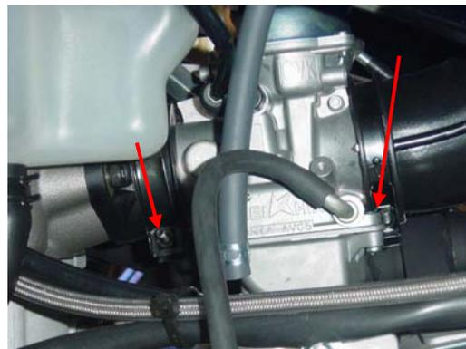
Loosen the all nuts on fixing studs and move all studs.
