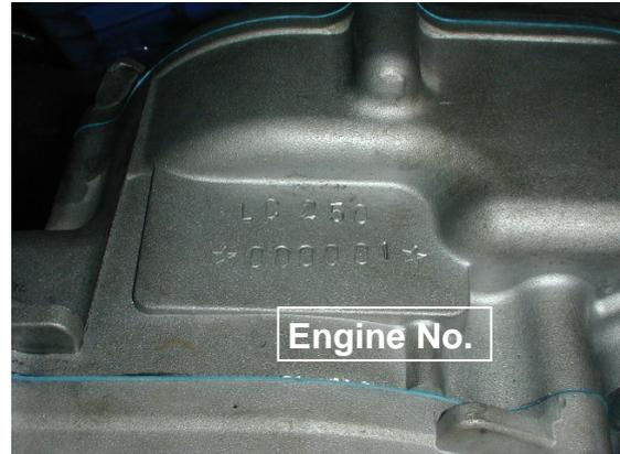
The engine serial number is stamped on the upper rear right crankcase.
