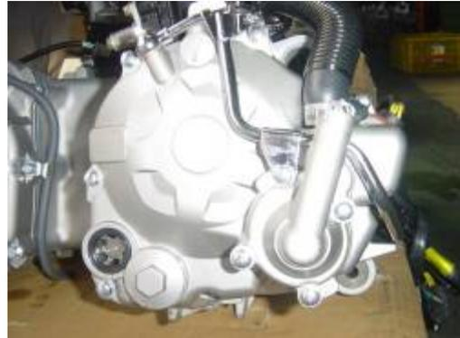
Remove the two pipe bolts, two 8 mm oil pipe bolts, 12 mm oil pipe bolt and washer, then remove the pipe.
