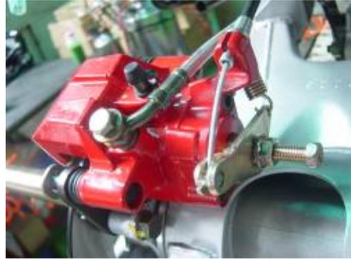
Installation is the reverse of removal. Using a C-clamp, depress the piston back into the caliper bore to provide enough room for the new pads to clear the disc.
