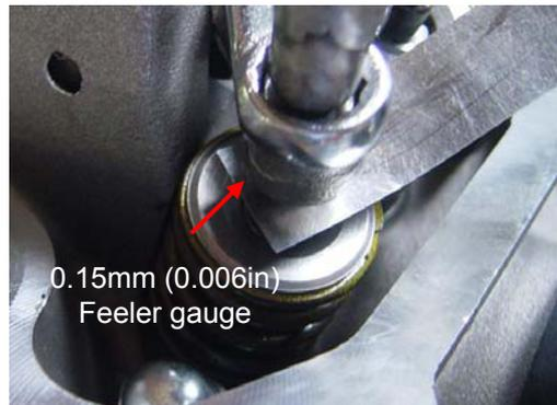
When the clearances are correct for all four valves, install the cylinder head cover.
