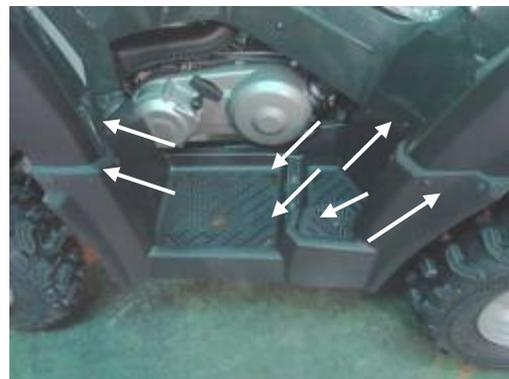
Remove upper fender to frame mounting bolts and front to rear fender joint bolts.
