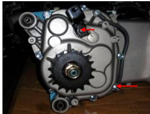
Remove gear shaft arm.
