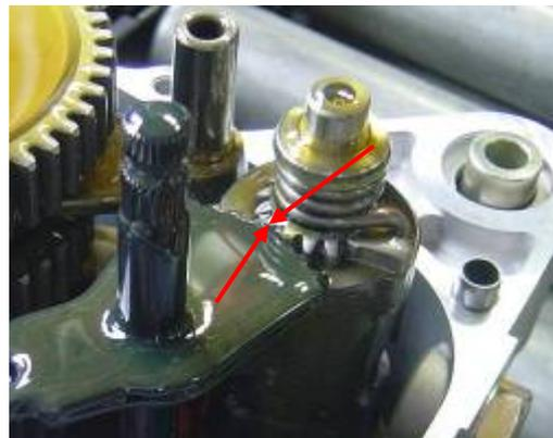
Install the dowel pins and a new gasket, add specified gear oil to gear box.
