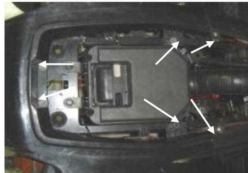
Raise up the fender and pull to back to remove the rear fender.
