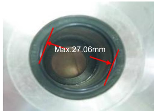
Check the drive face collar for wear or damage.
