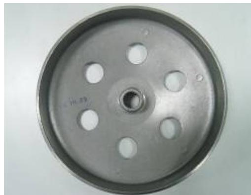
Check the clutch shoes for wear or damage.
