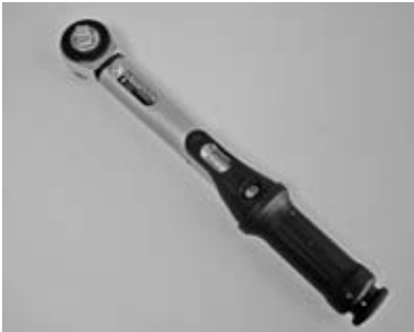
Torque wrench, measurement range 5 – 50 Nm
