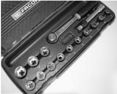
Reversible ratchet handle wrench and sockets, sizes 8 mm - 21 mm
