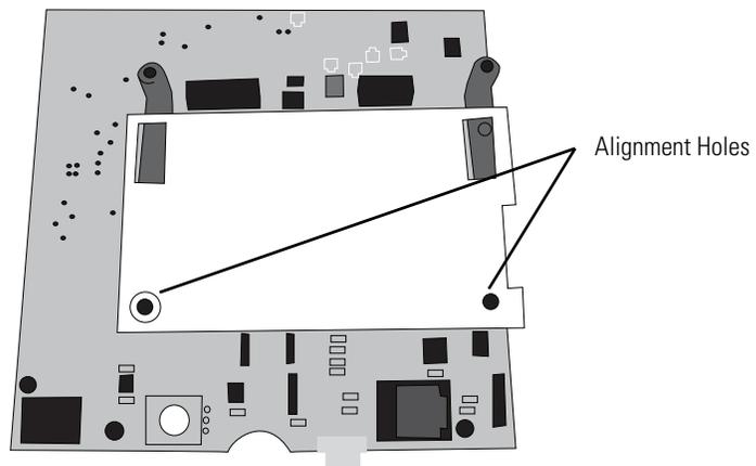
When reassembling, lay the shielding on top of the insulating paper and then replace the board. Verify shielding lays over top of standoff after folding.
