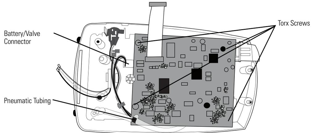
2. Remove the battery/valve cable connector from the bottom of the PCB.
