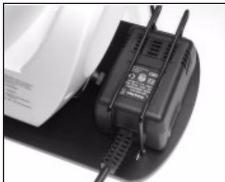
7. Replace the screw and firmly tighten it down so that the clamp is secure.
