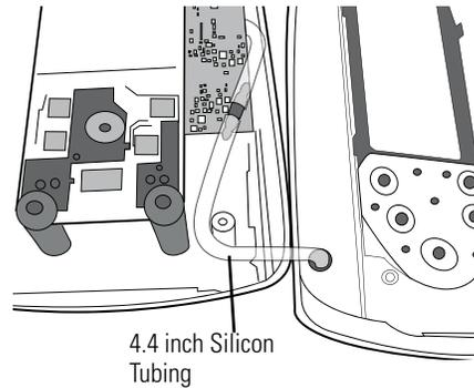
3. Insert one of the 1.5 inch silicon tubing pieces onto the "T" fitting.
