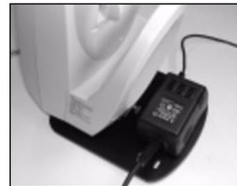
6. Place the wire clamp over the transformer and hook the two ends into the slots. The ends must slip underneath the plate.
