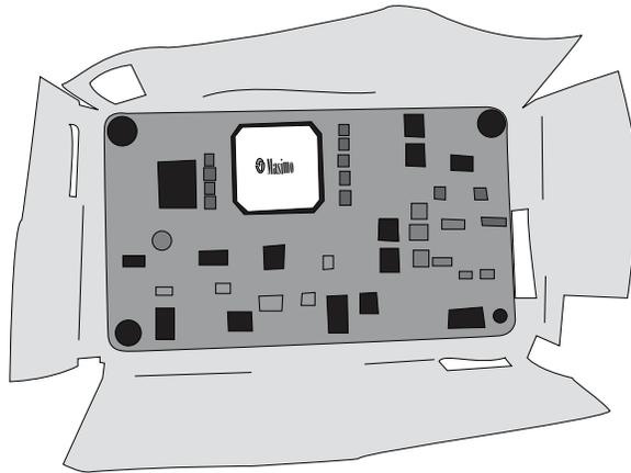
4. Remove the 2 screws and lift the board and shielding off the standoffs. This exposes insulating paper.
