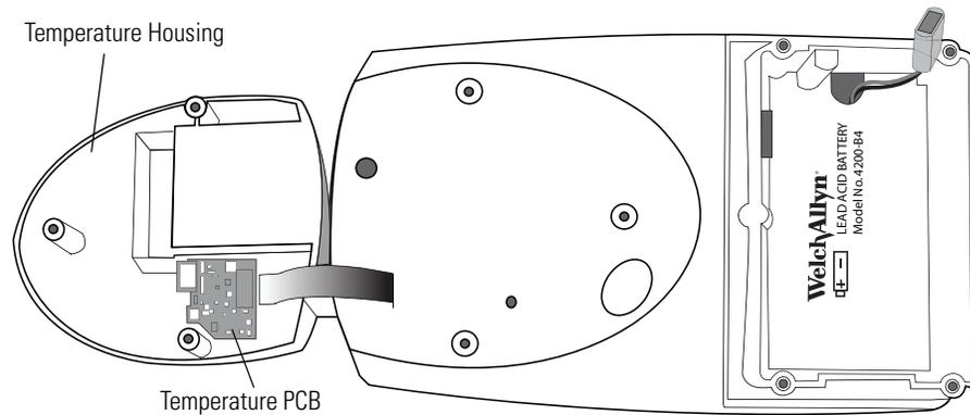
3. Unplug the flex cable from the connector on the temperature PCB.
