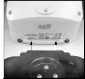
2. Slide the Spot Vital Signs onto the mounting plate and start integral screw into brass nut located on the back of the Spot unit.
