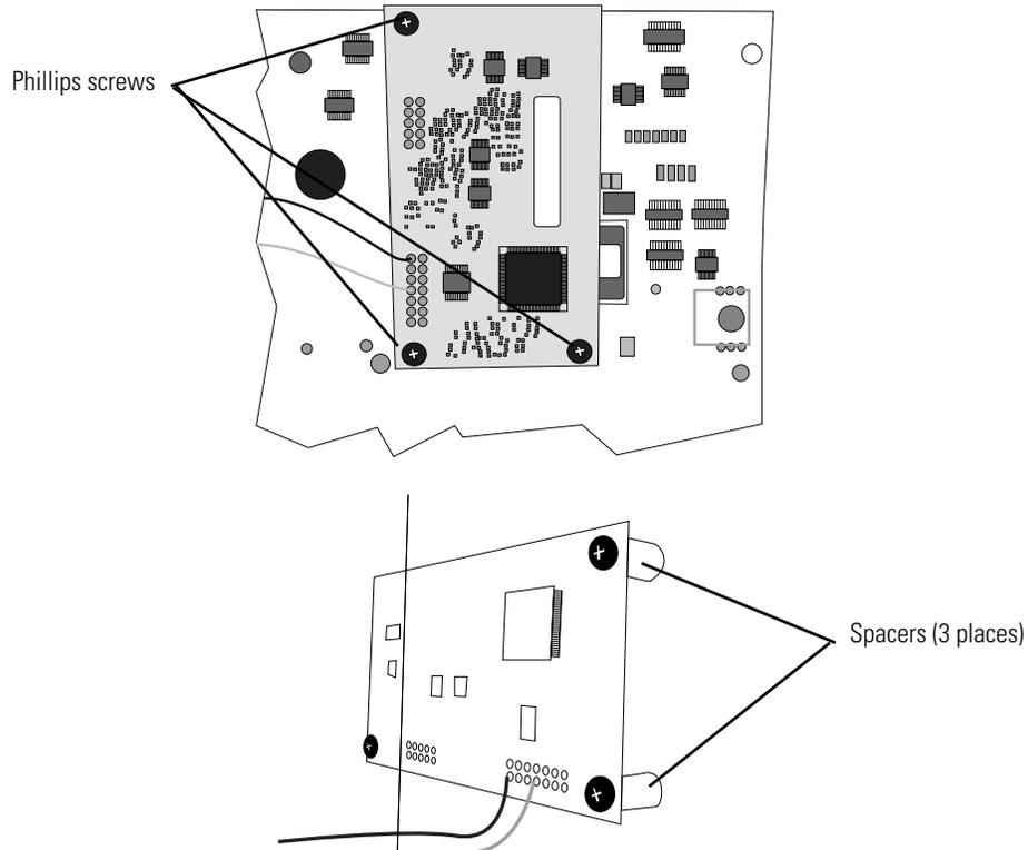
2. Remove the SpO<sub>2</sub> module (Nellcor MP205) from the main PCB.
