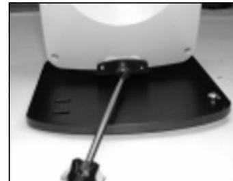
4. Remove the wire clamp screw and save it for later use.
