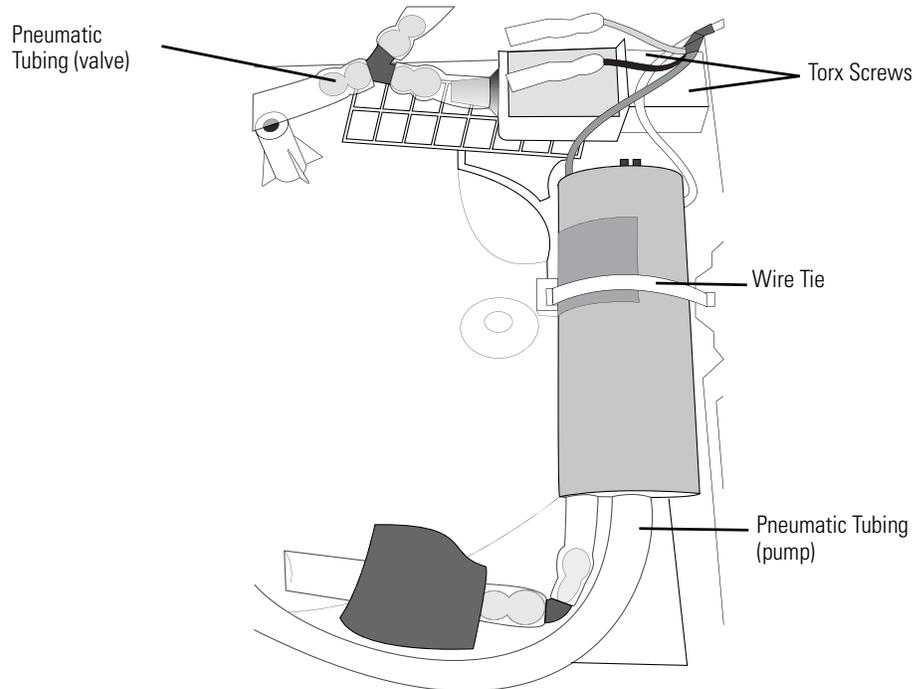
2. Cut the wire tie and remove the two Torx screws.
