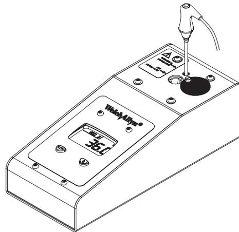
4. Wait for approximately one minute or until temperature on the thermometer is stable for ten seconds. Compare the thermometer's temperature reading to the 9600 Plus Calibration Set Point Temperature. If the temperatures are within  $\pm 0.1^{\circ}\text{C}$  ( $\pm 0.2^{\circ}\text{F}$ ), the thermometer is within calibration.
