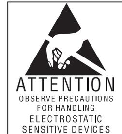
Electrostatic discharge is a sudden current flowing from a charged object to another object or to ground. Electrostatic charges can accumulate on common items such as foam drinking cups, cellophane tape, synthetic clothing, untreated foam packaging material, and untreated plastic bags and work folders, to name only a few.
