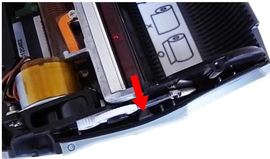
2. Take the interior mechanism from the printer bottom cover.
