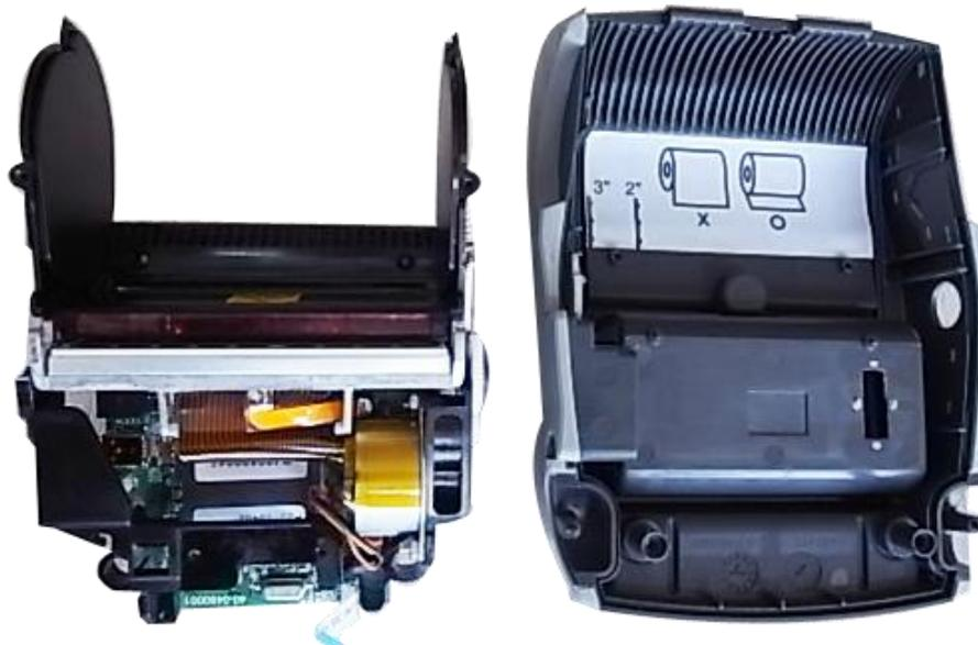
3. Plug the media holder adjustment knob to rotate the media holder to the closest position and remove a screw on the other side.
