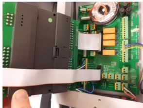
The DUC is now attached to the board by 2 ribbon cables only.
