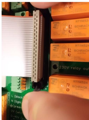
The spring locks on the plugs of the DUC's ribbon cables make it easy to loosen them from the circuit board.
