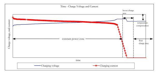
Battery current is controlled in a way to keep stable the power transferred to batteries in fixed power zone. If the voltage passes a certain value, balance charging starts. It is applied fixed voltage14.4V per battery (2.4V per cell). Boost charging takes 30 minutes. Then it passes to float charging. During the float charging, it is applied fixed voltage 13.5V per battery (2.25V per cell) in 25 °C environment temperature. UPS stays in this zone until the battery mode operation starts.
