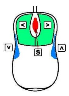
The optional mouse controller allows easy desktop access to the most commonly used front panel controls. These buttons are functionally equivalent to the corresponding front panel controls.
