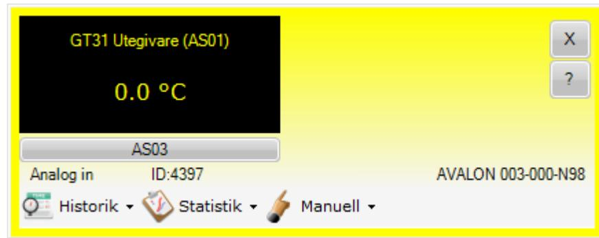
Analog in objects represent measured temperatures, pressure, moisture etc.
