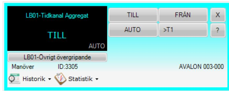
Maneuver objects represent fan control, pump control, the overall control for entire units etc.
