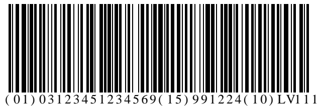
Figure 7-1 Example of a GS1-128 Representing a GTIN, a Best Before Date, and a Batch Number
