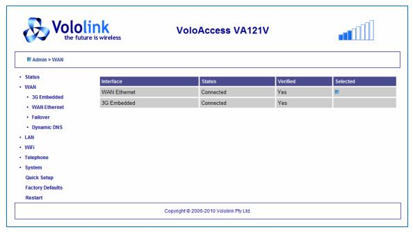
Observe the Connection and Verification status of the WAN interfaces. When all interfaces are fully operational, they are shown as being Connected and Verified with the primary interface Selected.
