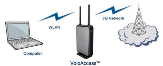
By default WiFi is Disabled. To set up a wireless network it is necessary to configure both the VoloAccess and the computer (or computers) that will be connecting wirelessly.
