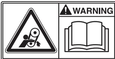
Belt drive: Keep hands, tools and other objects away from the belt drive when the machine is on to avoid injury and damage. See the safety instructions in the manual.
