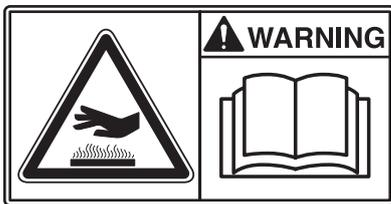
Engine, silencer: to avoid burns or discomfort, do not touch hot engine parts when the engine is on or when the machine has recently been used.
