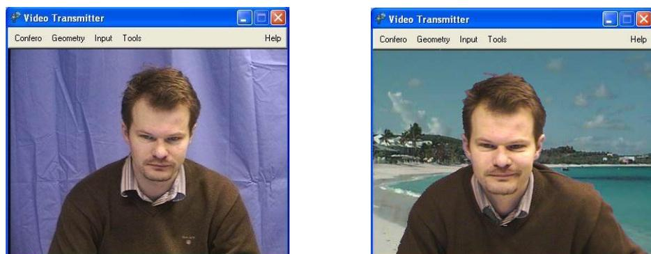
Figure 14. A chroma keying operation is performed on the video signal to the left, substituting the blue background with a still image showing a beach.
