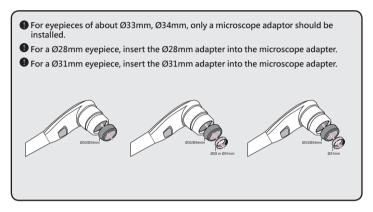
4. Mount / take off the microscope adapter onto / off the lens by doing the action shown in the picture.
