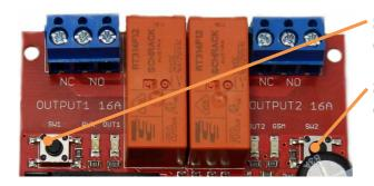
**SW1 Push Button:** Use for manual control of the Output1 relay.
