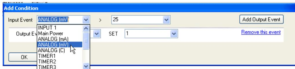
2. Click on the relational symbol to open up a drop-down box that allows you to select whether you want the **STP Sense** to react upon receiving an input greater than, equal to, or less than a specified value.
