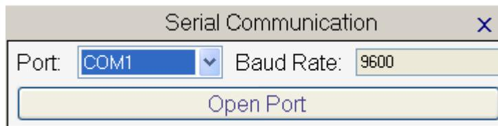
2. If there are several serial ports on your computer, select the appropriate one from the drop-down list near **Port:**, and type in the Baud Rate.
