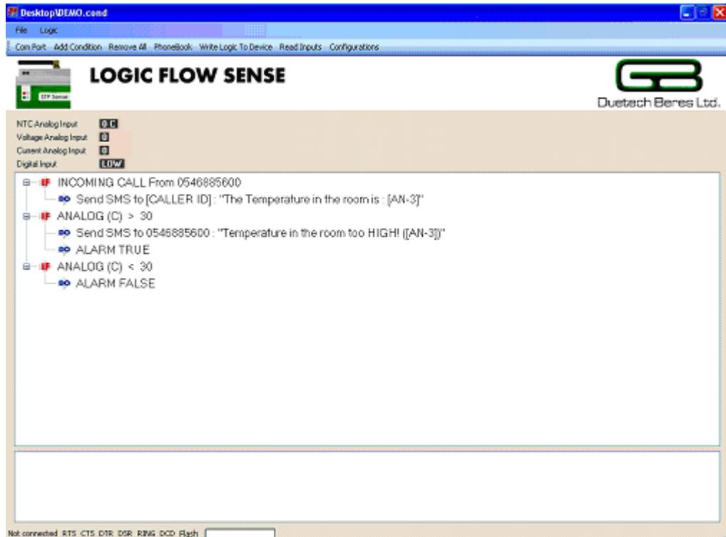
21. After creating all the logic conditions, click on **Write Logic to Device** in the main toolbar.
