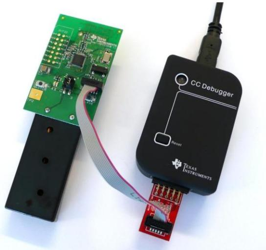
**Figure 7: CC Debugger + SmartRFCCxx10TB**
