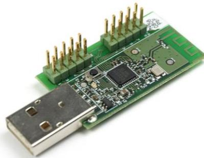
Figure 5: CC2511/CC1111 USB Dongle
