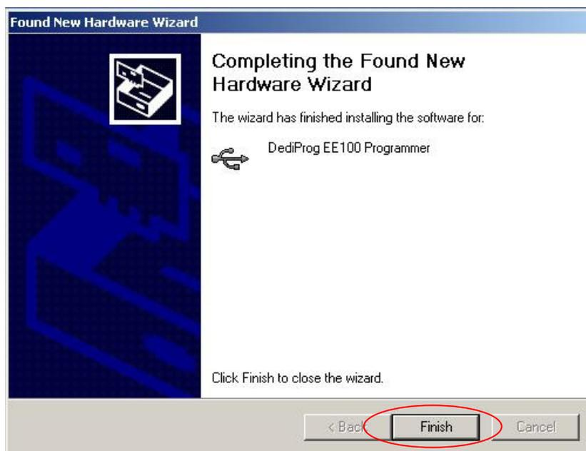
If the USB driver is installed properly, users can find “Dediprogram EE100 Programmer driver” under device manager when the programmer is plugged into the PC.
