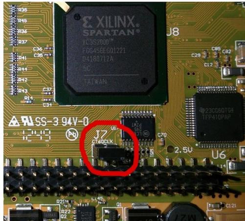
Only **one** such filter is allowed to be enabled on any board stacked on the CT60.
