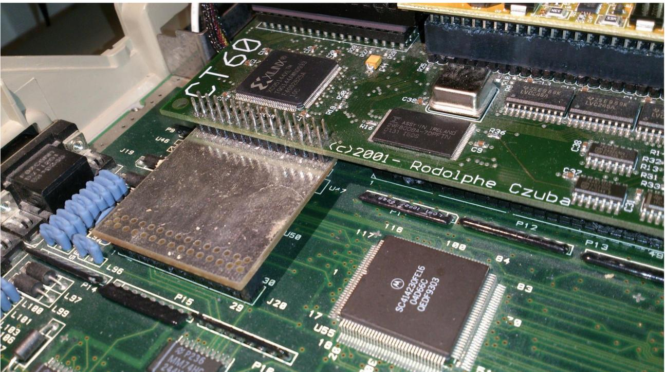
Note that this shows a prototype of the Extender boards, hence the silver colour. Also note that the longer Extender is hidden below the CT60.
