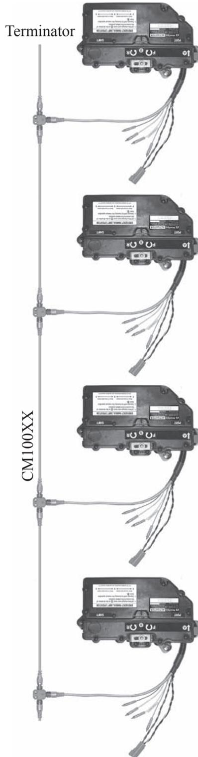
*Note: Actuators may be added to the CAN Bus in any order or in any location.*
