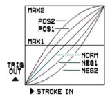
The Max1 and Max2 setting result in a fixed -6 resp. 0 dB trig level.
