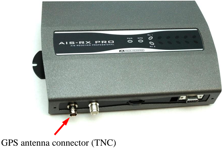
Figure 3 GPS antenna connection
