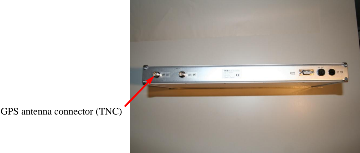
Figure 4 GPS antenna connection
