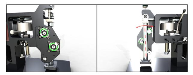
4. Verify that the measuring plate is correctly adjusted and repeat the adjustments with the gauge blocks if necessary.
