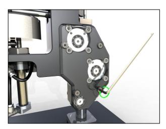
2. To adjust misalignment between front and rear of the measuring plate, loosen the 8 screws that hold the eccentric adjustable linear unit.
