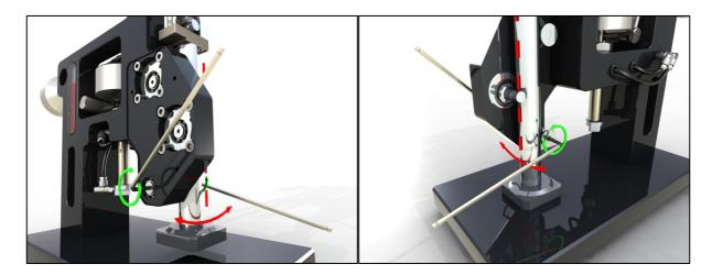
3. To adjust misalignment between the sides of the measuring plate, tighten or loosen the lower alignment bearing with the use of two hex socket wrenches. The position is spring loaded and no additional fixation is necessary.
