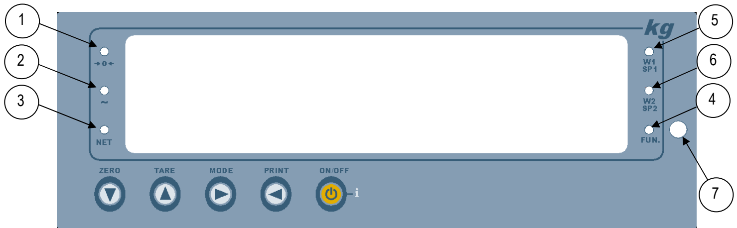
Figure 6.3 – Keys and indicators of the DGT60 front panel
