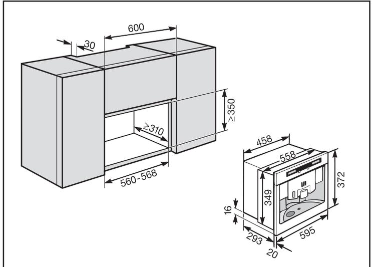
It can also be combined with other Miele built-in appliances. If the coffee machine is to be built in above another appliance, there must be a full-width, closed shelf between them (except when it is combined with a Miele built-in plate warming drawer).
