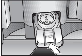
Put the coloured descaling funnel in its place.
