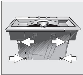
If this is not the case you can adjust the height of the 4 feet underneath the machine using the large spanner.
