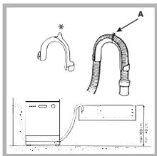
The special plastic elbow\* makes it easier to find the best layout: fix the elbow to the wall securely in order to prevent the outlet hose from moving and spilling the dirty water. The part of the hose marked with the letter A should be between 40 and 100 cm above the ground (see
