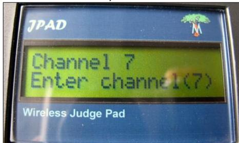
3. Enter the Channel (0 to 9 – Default is 7), and press Send (>) button to confirm.
