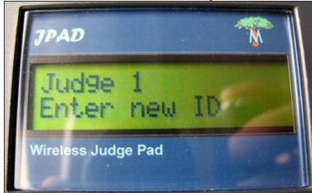
2. Enter the ID required, and press Send (>) button to confirm and see the Channel menu;
