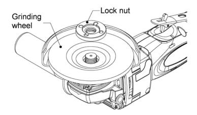
Pressed the fixed button after tighten the lock nut. Use the spanner to tighten the lock nut completely.
