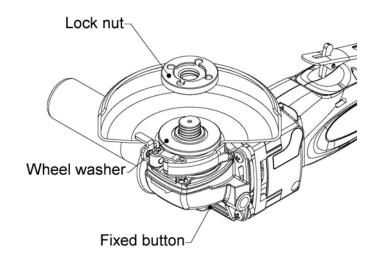
Place the grinding wheel on the wheel washer tighten the lock nut by hand.
