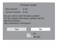
DO NOT DISCONNECT the unit from the AC power or perform any operation while the update takes place.
