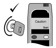
**5C** If "Lockout 0:60" is displayed on the LCD and the status LED is solid red, you have exceeded the 0.20‰ BrAC limit. You cannot start the vehicle.
