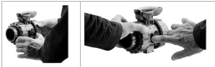
Fig. 11: Unlocking union nuts
