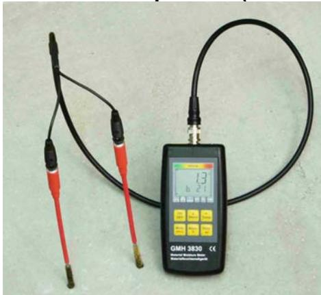
**Measuring concrete with brush probe HND-FF06**
