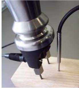
**Reciprocating piston electrode HND-FF01 with temperature-probe –FF10**
