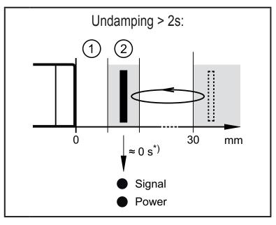
If the target was away from the sensor for less than 2 s (> 30 mm), the yellow LED comes on without delay in case of damping in the enable zone.
