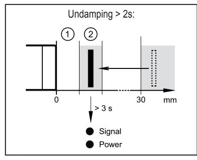
If the target was away from the sensor for more than approx. 2 s (> 30 mm), the yellow LED goes on with a delay of approx. 3 s in case of damping in the enable zone.
