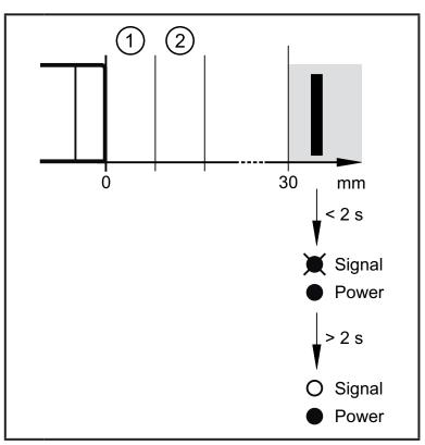
If the sensor is undamped for more than 2 s (> 30 mm), the adjustment mode is switched off and the yellow LED goes out.
