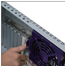
5.1 Push out to loosen add on card kit
