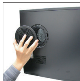
Easy-clean filter (in left side panel)
