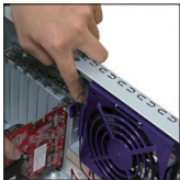
Screw-less Add-on Card assembly
