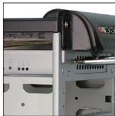
6.2 Unscrew the screws holding the floppy cage
