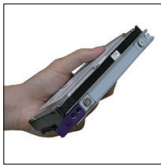
3.2 Attach rails to both sides of your HDD
