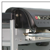
6.7 Secure the floppy cage by screws
