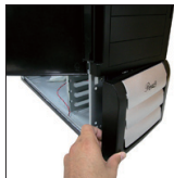
8.1 Push front panel hooks to detach the front panel from the chassis ( please refer to step 1.4 )
