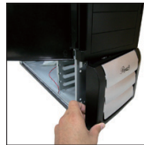
Easy-clean filter (in front panel)
