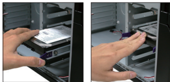
3.3 Insert the railed HDD into the 3.25" HDD bay and push to the bottom
