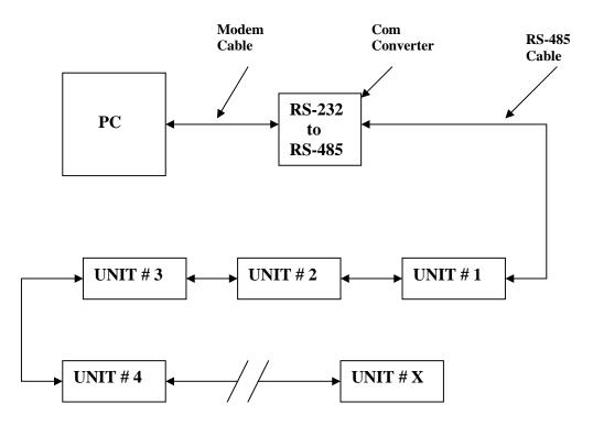
Modem cable – generally, a 9 pin M to a 9 pin F, straight-through cable, depending upon the PC's com port, and the communication converter's RS-232 port.
