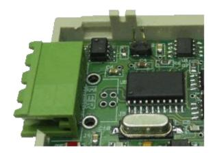
When a jumper link is fitted, autoreverse operation is enabled:
