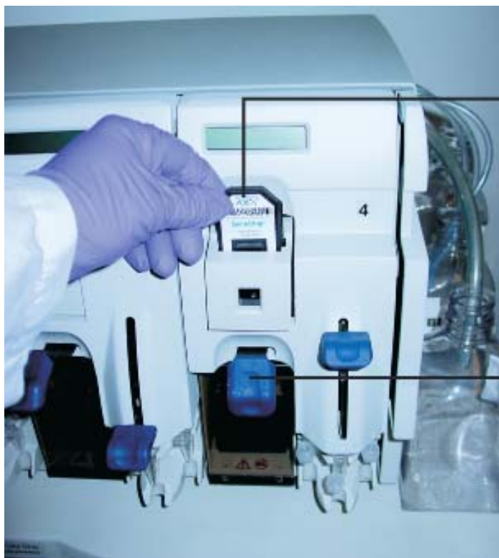
Figure 7.1 Disengaged washblocks showing cartridge levers in the down position. Remove any cartridges
