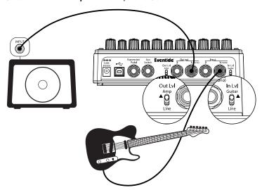
This is the simplest way to connect SPACE. Connect your guitar cable to SPACE Input 1 and a cable from SPACE Output 1 to your amp. Input and Output Level switches (In Lvl & Out Lvl) should be set to GUITAR and AMP.
