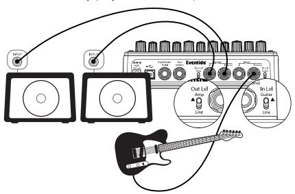
Connect your guitar cable to SPACE Input 1 and a cable from SPACE Output 1 to one amp and a second cable from SPACE Output 2 to the other amp. Input Level switch (In Lvl) should be set to GUITAR and Output Level switch (Out Lvl) set to AMP.
