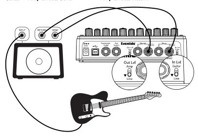
If your Amp has an Effects Loop, you can connect SPACE's Input to the Amp Effect Loop Send and SPACE's Output to the Amp Effect Loop Return. Most guitar amp's Effects Loops run at Line Level so set SPACE's Input and Output Level Switches to "Line."
