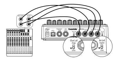
When connecting SPACE to a Mixer, set SPACE's Input and Output Level Switches to "Line."
