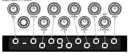
Since any number of parameters can be programmed to respond to the pedal, it's important to learn how to un-assign parameters. Let's say that you've programmed the Pedal to control Mix from 50% to 100% and Delay from 10 milliseconds to 100 milliseconds. Now, you'd like to unassign Delay and have it fixed at 20 milliseconds rather than have it change when the Pedal moves. Here's what you do:
