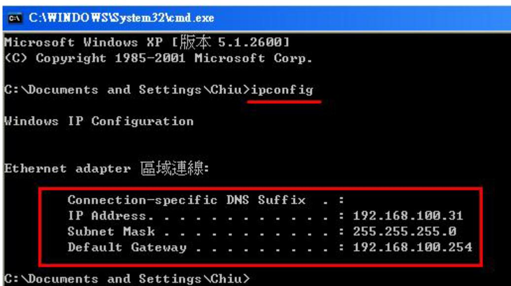
IP 9060(A) Default static dynamic IP Address is **192.168.0.100**. **the last digit of IP address (default is 100) can be any number between 1~254, but can not be same as your PC.**
