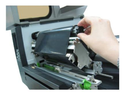
6. Ensure the ribbon is as tight as possible. Push down the print head unit so it locks under the green catch at the front.
