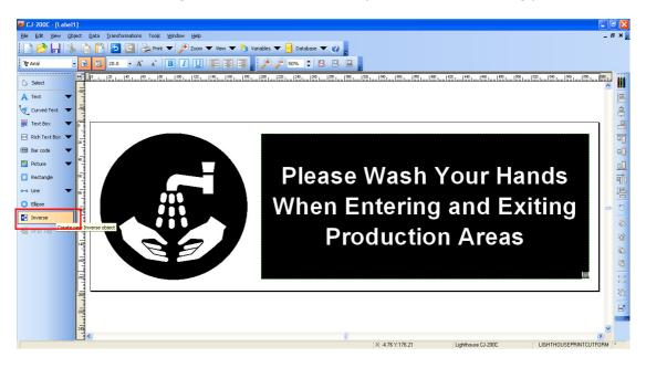
As the CJ200C is a thermal printer, it uses heat to transfer the ribbon into the vinyl. When inverse printing, it is recommended that the darkness setting is reduced.
