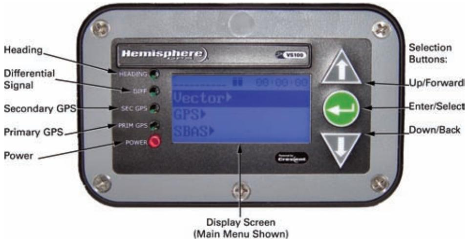
**Figure 5-1. LED Indicators, Display Screen and Selection Buttons**
