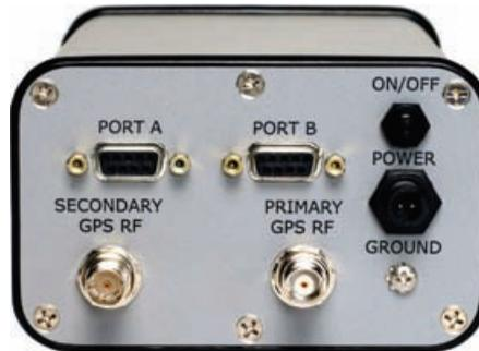
**Figure 3-4. Port connections on the VS100 Series.**
