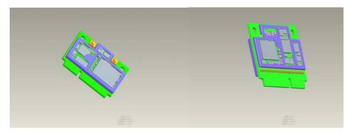
All components except the two antenna connectors are covered by EMC shields. All power and communication is routed through the edge connector of the card. The fastening holes in the upper corners are connected to ground.
