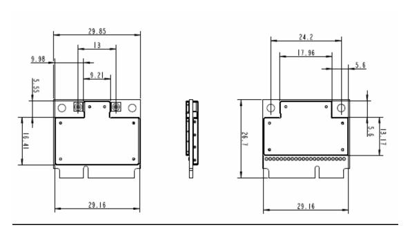
There are three connectors located on each card: two RF connectors located in the top corners and one system connector located on the lower edge.
